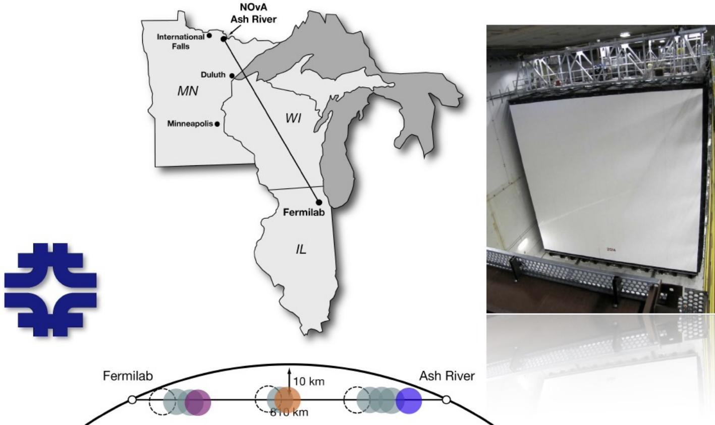
14,000-ton surface far detector sited at first oscillation maximum.
