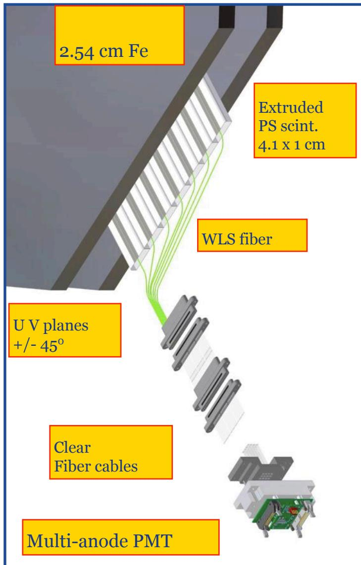
Steel thickness: 2.54 cm ( $\sim 1.4$  rad. lengths)
