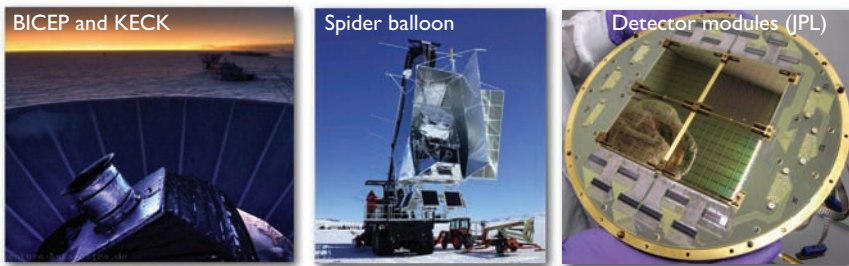
Fig. 6. The BICEP telescope with the Keck ground shield in the background, the Spider balloon-borne telescope, and an image of the planar array detector modules they employ.
