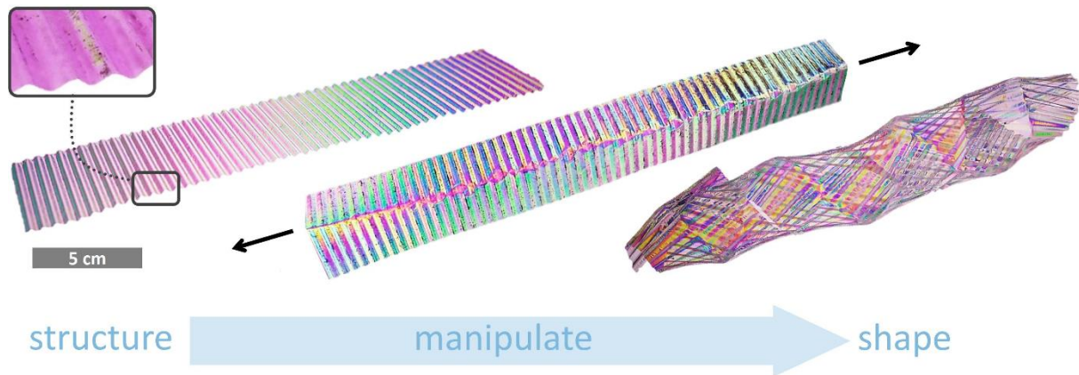
Figure: An undulating origami sheet undergoes a rapid, elastic snap-through transition to a new stable configuration when edge point loads are applied. Viewing the structure between crossed polarizers emphasizes the difference between the two stable shapes via optical birefringence of the sheet material.
