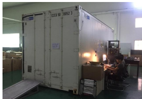
Batch test of 36 PMTs within a container
